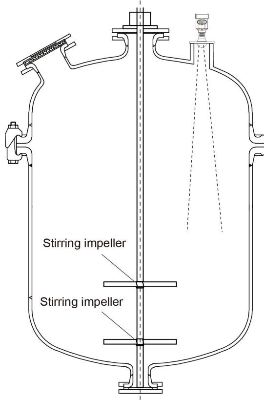
Remarks: Cannot be installed above the inlet, there can be no obstacles under the meter
