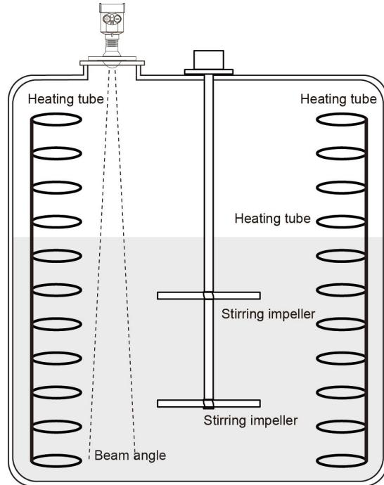
Extremely low emission angles ensure accurate measurements under extreme conditions
