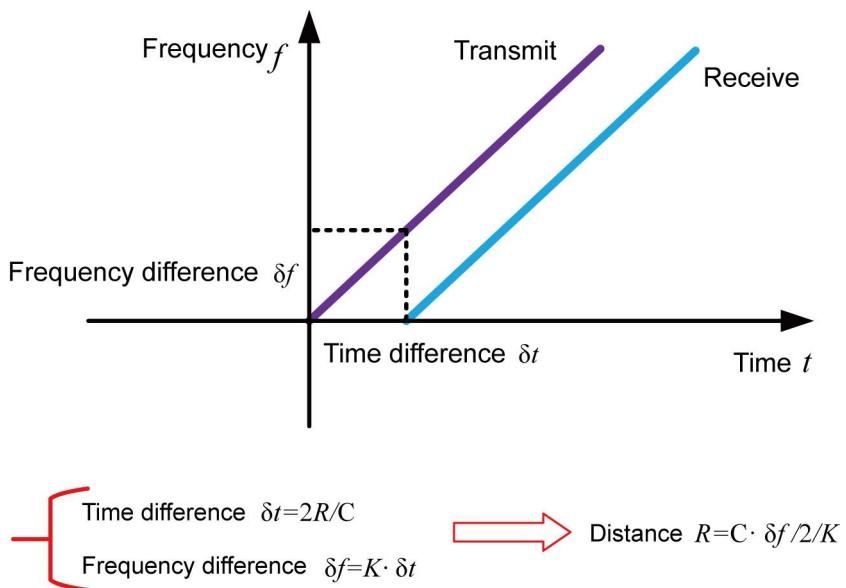
Note:  $K$  is the frequency modulation slope
